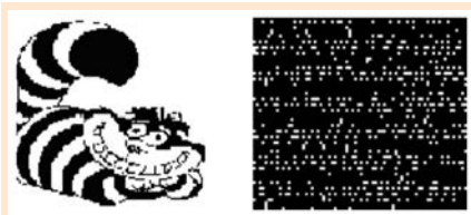
Figure 4. The Cheshire cat (128 × 128 pixels) and a small part of its CGH.
