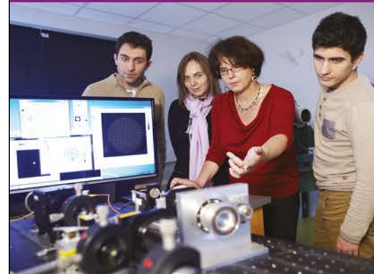
Figure 2. Two applications in quantum optics for the measurement of photon correlations. In the case of time correlations the aim is to characterise a single photon source based on a quantum dot [2] operating in the pulsed regime. In this case, it is the absence of a correlation peak at \tau = 0 which is significant. It reflects the fact that two photons are never produced simultaneously by the source. Conversely, the presence of correlation peaks at \tau \neq 0 is interpreted as the probabilities that a second single photon will be emitted in the next or previous pulses. Typically, it is the ratio of the two peaks (central to lateral) which enables the quality of a single photon source to be determined. In the spatial case, we introduce boson sampling, which consists in calculating the spatial correlations of a pair of photons at the output of a network of coupled waveguides of dimension k \times k in which the coupling between the guides enables the action of beamsplitters to be simulated [3]. In this case correlated detection of photons is essential, since it enables the pairs of photons which actually travelled together (i.e. in the form of a two-photon wave packet) to be distinguished from those which travelled independently of one another (in the form of two single-photon wave packets). In fact the spatial signature at the output of the network in the two cases differs greatly, due to two-photon interference, which has no conventional equivalent.
